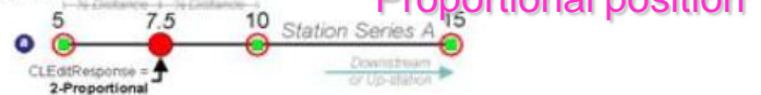
a – Three control points are located on a single PRM station series (A). A single point OnlineFeature with a CLEditResponse = 2 is located at station value 7.5 which places it ½ way between the control points with station value 5 and 10 respectively.
